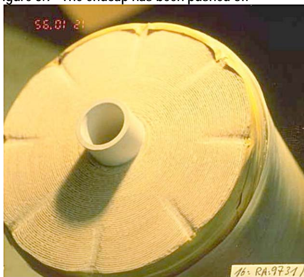
Figure 8.9 The endcap has been pushed off
