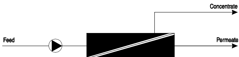
Figure 3.1 Continuous RO process
