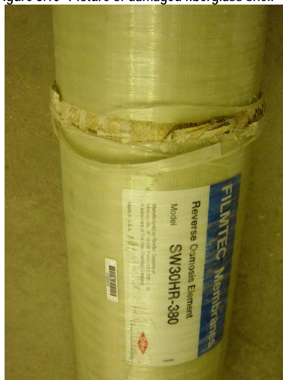
Figure 8.10 Picture of damaged fiberglass shell
